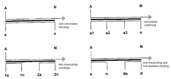
One end of the primary winding is insulated from ground, and the second one is grounded during operation. One secondary terminal of each output must be grounded before putting into operation.
